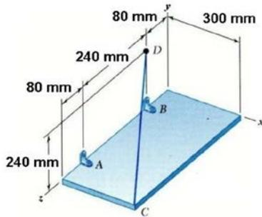
GIVEN: A shelf is supported by two brackets and a wire (CD). The tension in the wire is 200N.
