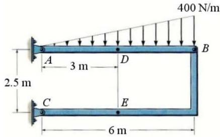
Determine the normal force, shear force and moment at a section passing through point D of the two-member frame.
