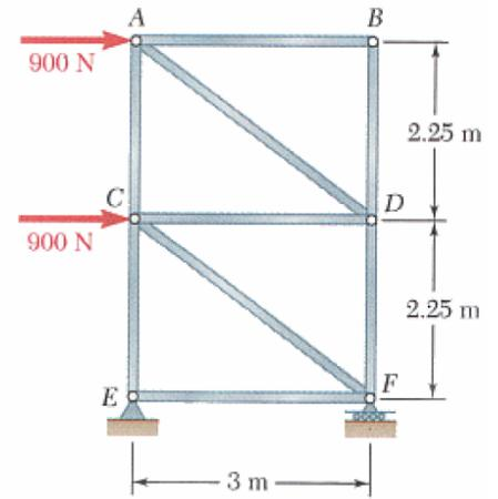
6-59. Determine the horizontal and vertical components of force at pin A.
