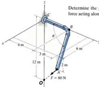
Determine the projected component of the 80-N force acting along the axis AB of the pipe.
