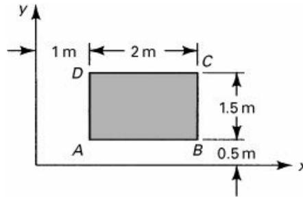
where  $c = 10^{-4}$ . Subsequent to the loading, determine (a) the length of the sides  $AB$  and  $AD$ ; (b) the change in the angle between sides  $AB$  and  $AD$ ; and (c) the coordinates of point  $A$ .
